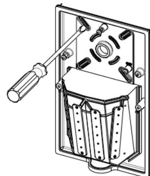
Step3: Using tools to open the installation position of Junctions Box, then fix the lamp on Junctions Box.
