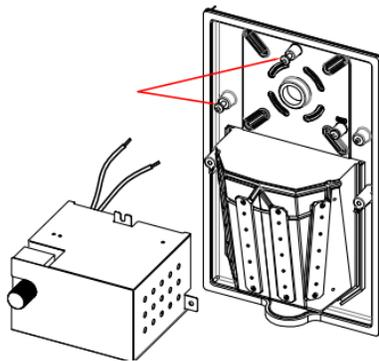
Step2: Loosening the two screws as shown in the picture, take off the driver box.
