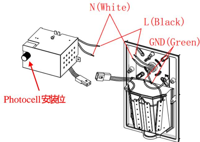
Step5: wiring, Line(Black), Neutral(White), GND(Green), see the below connection diagram, connect the connector between the power and the led board.
