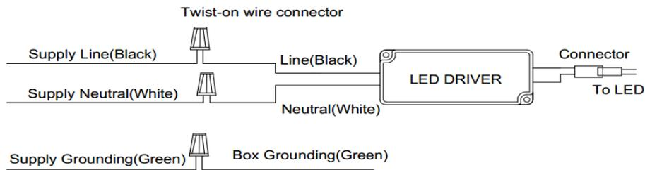
Wiring layout without Photocell
