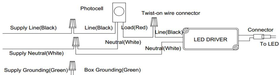
Wiring layout with Photocell
